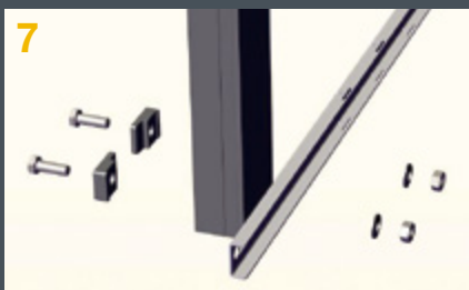
7 Another cross beam is attached in the shaft pit.
