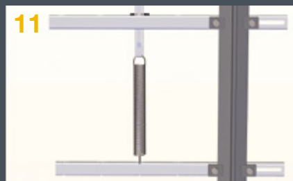
11 The tape suspension is hooked on the tension spring.
