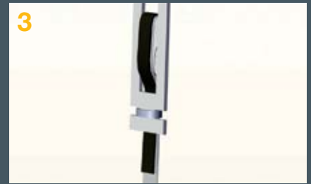
3 The magnetic tape is inserted in the tape suspension.
