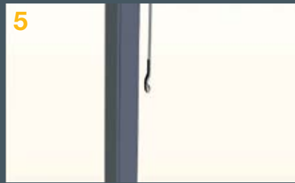
4 Standing on the car roof, the magnetic tape is rolled out during the ride down and inserted at the lower end in the tape suspension.
