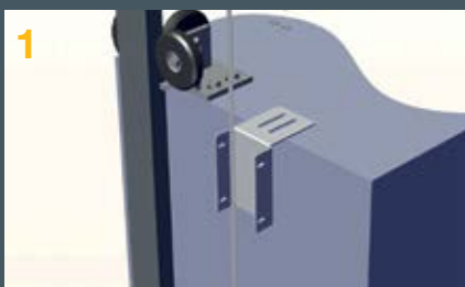
1 The sensor is mounted on the car using a mounting bracket and connected to the controller or SAFE BOX via cable.
