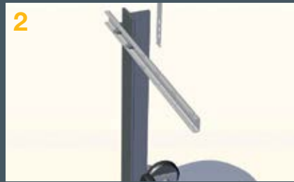
1 A cross beam is mounted at the upper end of the shaft on the elevator guiding rail.
