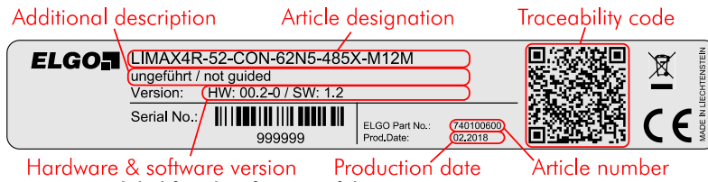
Fig. 3: Type label for identification of the sensor
