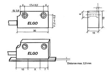
Over the distance X, the gap between sensor and measuring tape must fall between 0,1 and 2,0 mm.
