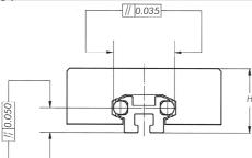
Guiding accuracy Install. height *H* - tolerance Deviation on one rail
