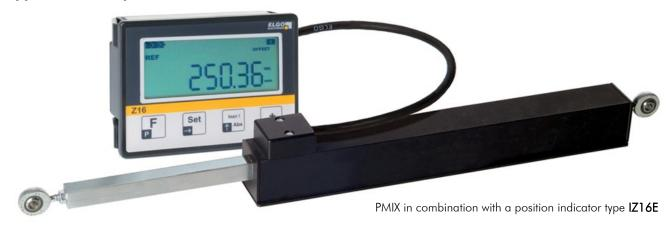
Depending on the ordered version, an LMIX, EMIX or EMIX23 sensor can be integrated in the PMIX housing. As shown in the photo above, the PMIX system can be combined with the battery-powered ELGO position indicators IZ14E, IZ15E, IZ16E and IZ17E. In this case sensor and resolution comply with the selected IZ unit. Further no wiring is necessary. The respective ordering suffix is specified in the type designation.
