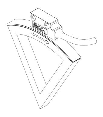
The magnetic tape is glued on a solid ground (e.g. angle stop) along the measuring distance.
