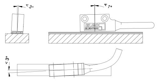
The cable must be laid in such a way that there is no risk of damage as tension or bruise. If necessary, use a drag-chain or a protective tube and provide a strain relief.
