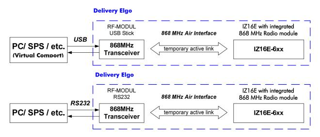
The IZ16E-600 and the 868MHz transceivers are equipped with powerful, integrated ceramic antennas. External antennas are not necessary.
