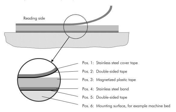
Figure 1: Components of the magnetic tape
