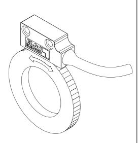
A pole ring / magnet wheel is mounted on a rotating axis (E.g. motor shaft).
