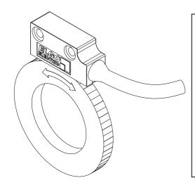
A pole ring / magnet wheel is mounted on a rotating axis.
