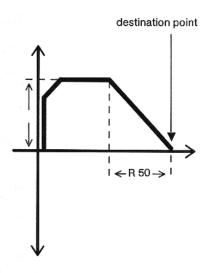
R 50: Set deceleration distance 0.1 to 999.9 mm by means of keypad
