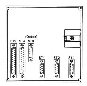
To activate signals, pull input down to zero volts. By changing internal optocoupler, positive logic is available ie pull input up to 24 v dc.
