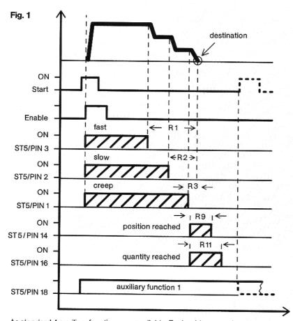
As standard 4 auxiliary functions are available. Each address can have one of these 4 selected. The output is energised so long as the address is selected, until the start for the next sentence is activated.
