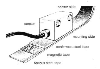
The tape is impervious to oil, dust, chips, and sawdust, allowing the magnetic sensor and tape to be installed in the most arduous machine and shop floor environments.
